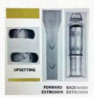
This cribsheet will focus on the central bursts in the product of cold drawn steel, especially from the point of view of a shop making parts on automated equipment.
