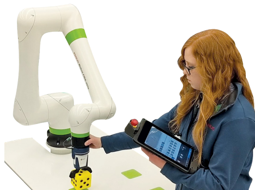
An operator teaches the CRX Collaborative Robot by guiding it manually.
