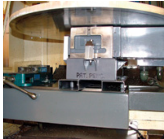
As part of its continuous improvement, Micromatics developed this indexing table so the company could use a mill as an assembly press.
