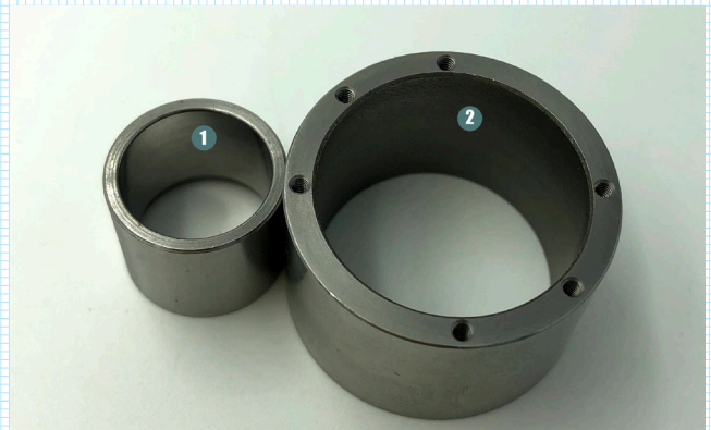
Item (1) shows an ID that has gone through a honing process for a polished finish. Item (2) shows a turned part with a standard finish on the ID.
