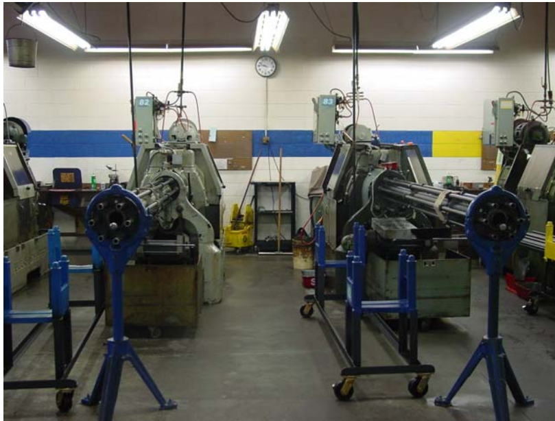
Color coded 9/16" Acme Gridley. Blue color indicates 9/16" Acme.
