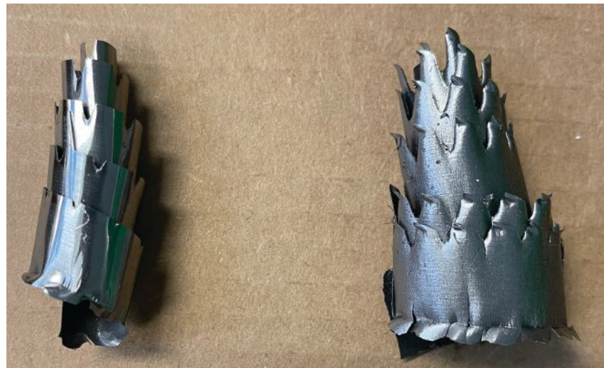
1215 Chip new tool (left) and end of tool life (right). Chips courtesy of Herker Industries Inc.
