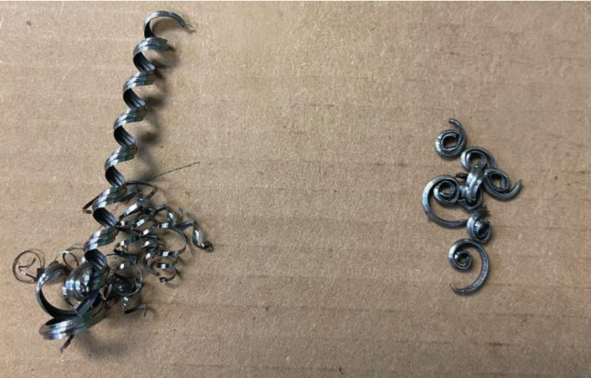
1020 DOM after tool change (left) and before tool change (right). Chips courtesy of Herker Industries Inc.
