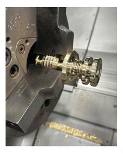
situation where the groove dimensions constrain the chip, contributing to the chip evacuation and massing problems we encounter with unleaded materials.
